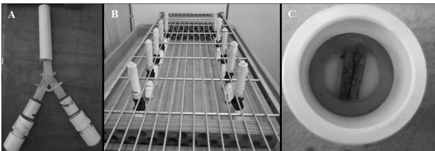
Fig. 3. Y-tube assay: (A) assembled Y-tube assay, (B) assays in frame in a controlled-environment room, (C) bottom cap with grape root pieces.
